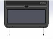
7. Remove protective cover and tape from front of display.
