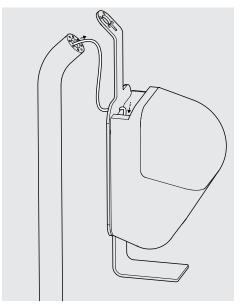
Feed power cable through Printer
