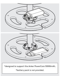
15.2 If installing a battery pack, connect the tablet cable and locate the pack into the Floorstanding Base.
