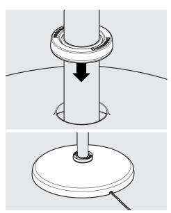
With the Floorstanding Cover on the ground, locate and fit the Floorstanding Rubber Collar.
