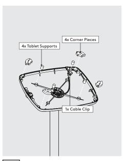
Install the Tablet Setup Kit. Each kit is specific per device & case.
