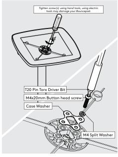
Locate and secure the Case onto the Mounting Arm as shown. Tighten by hand.
