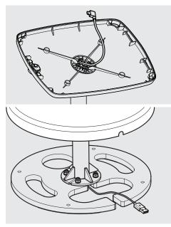
Feed the tablet power cable through the Case & Floorstanding Pole.
